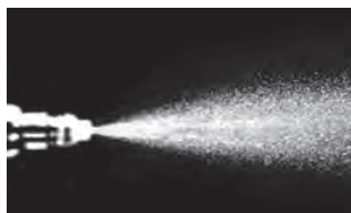
Injector spray pattern after P.i. treatment.
